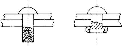
Figure 1.48 Explosive rivet
