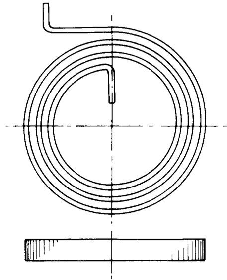
Figure 1.74 Spiral torsion spring (rectangular section)
