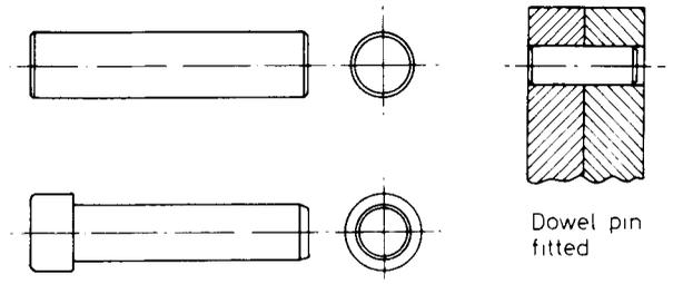
Figure 1.50 Dowel pins
