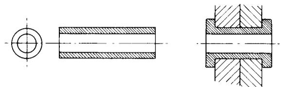
Figure 1.46 Tubular rivet
