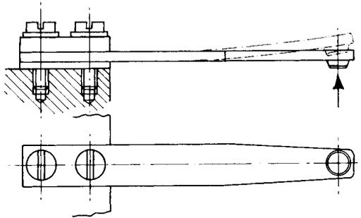
Figure 1.78 Cantilever leaf spring (electrical contact)
