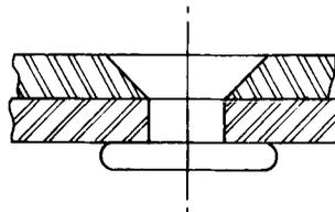
Figure 1.45 Flush rivet
