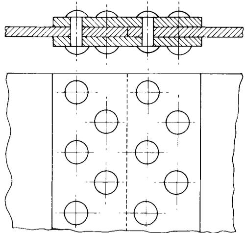
Figure 1.44 Double riveted butt joint with two straps
