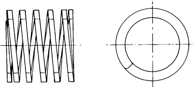
Figure 1.70 Rectangular-section spring
