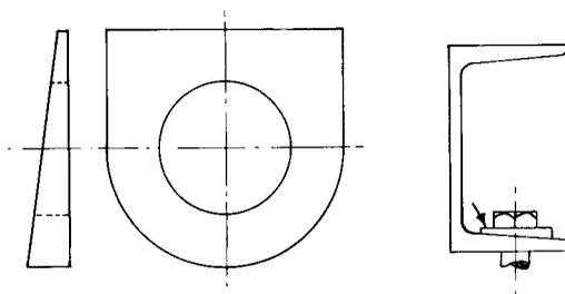
Figure 1.37 Taper washer and application
