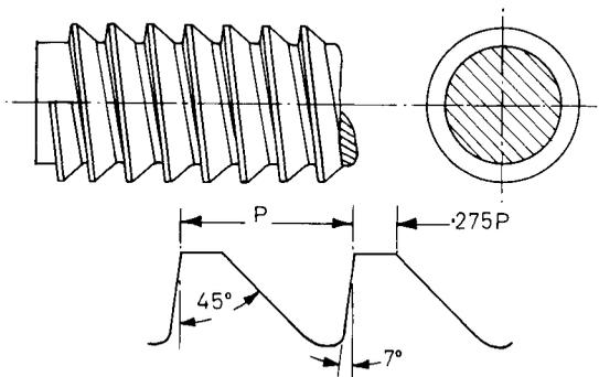
Figure 1.66 Buttress thread
