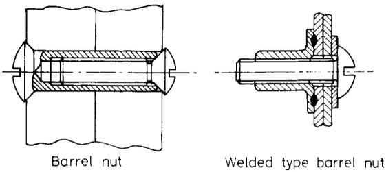
Figure 1.28 Barrel nuts
